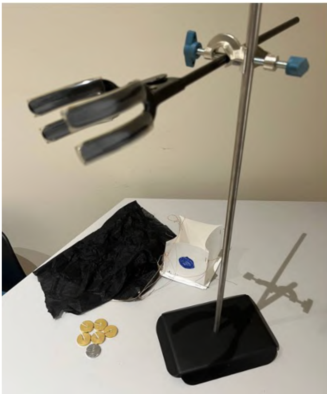
Figure 1. This paper's materials include a retort stand, meter ruler, masses, and a do-it-yourself parachute made from cloth and cloth tread.
