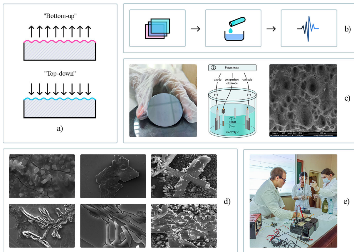
Figure 1. Nanomaterial synthesis: a) approaches to nanostructure synthesis; b) and c) scheme of electrochemical dissolution of crystal; d) examples of synthesized nanostructures; e) master-class “Chemistry? Alchemy? – No. Electrochemistry!”.
