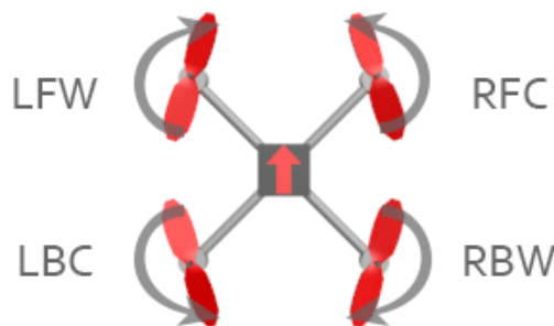
Fig.1 Direction of rotation of the screws and location of the motors.
