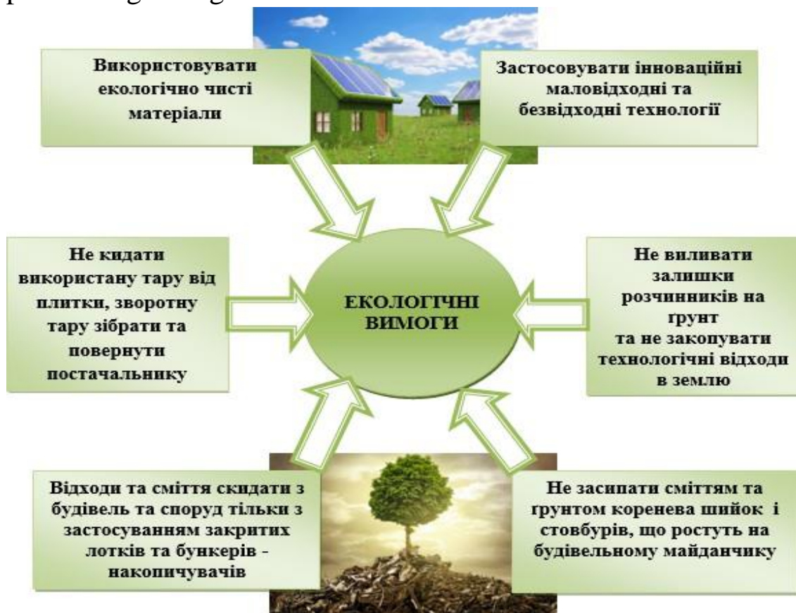
Fig. 3. Ecological requirements for the execution of facing works (developed by the author)
